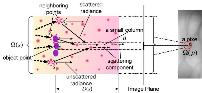
**Figure 8.** Schematic representation of the effect of scattered radiation and the finger-vein image degradation process. Here, both  $s$  and  $p$  respectively corresponds to any one point in  $x$ - $y$  coordinates.
