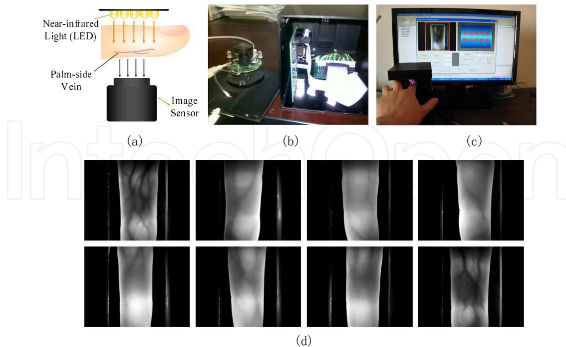
**Figure 1.** Finger-vein image acquisition. (a) NIR light transillumination. (b) A homemade finger-vein imaging device. (c) Our finger-vein image acquisition system. (d) Some captured finger-vein images.
