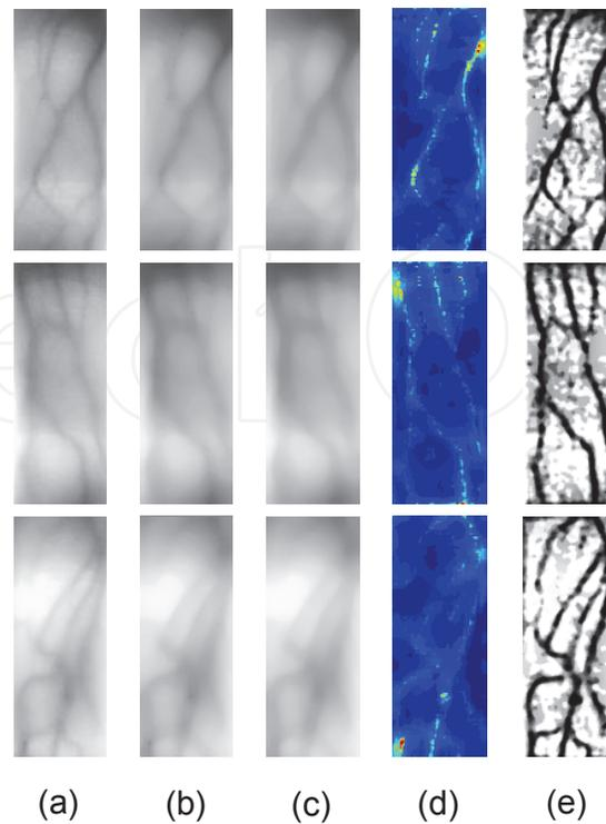
**Figure 10.** Scattering removal experiments. (a) Some captured finger-vein images  $I(x, y)$ . (b) The estimated scattering components  $V(x, y)$ . (c) The estimated scattering radiations  $I_r(x, y)$ . (d) The estimated transmission maps  $T(x, y)$ . (e) The restored images  $I_0(x, y)$ .
