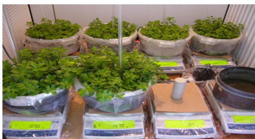
Figure 1. Weighing balance for transpiration measurements
