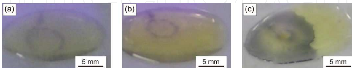
Figure 13. Picture of nanoparticle structures for (a) R_m = 1 , (b) R_m = 2 , and (c) R_m = 10 . I_D=2 mA, P_{gas}=20 Pa, B_{IL}=1 T.
