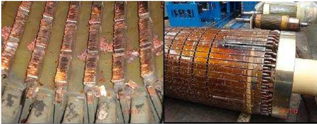
Figure 26. Stator and Rotor Damages
