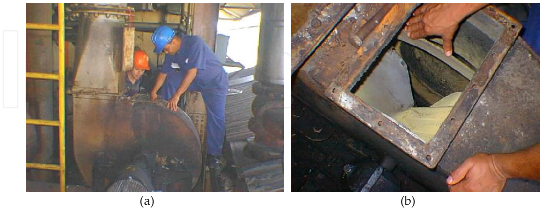
Figure 7. Photos of the attack-sites of samples: a) Ventilator extractor where samples were placed, b) Ventilator damp where samples were anchored.
