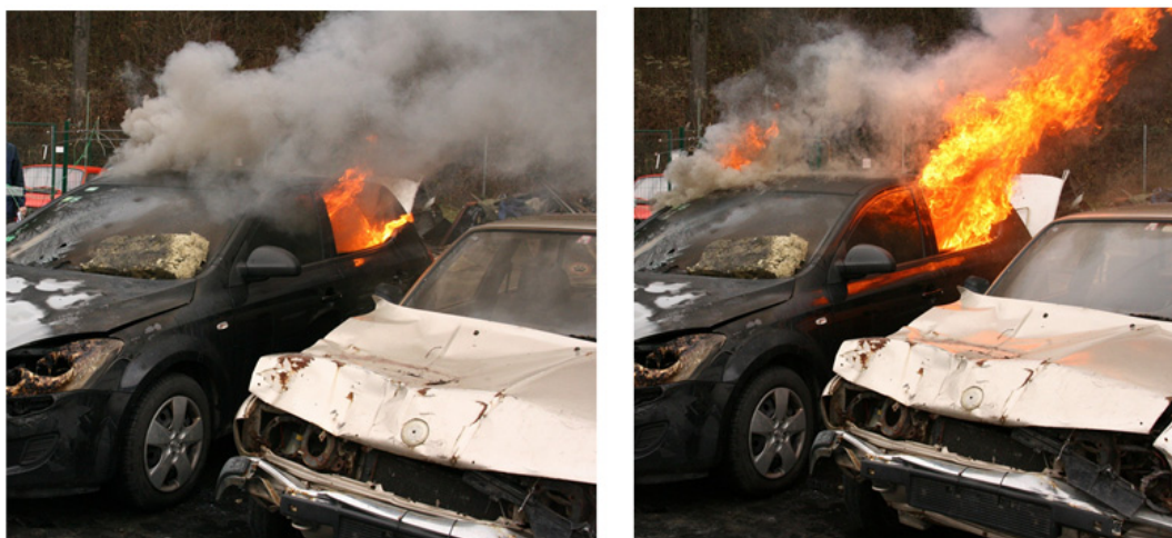
Figure 12. Full-scale fire experiment: passenger compartment fire
