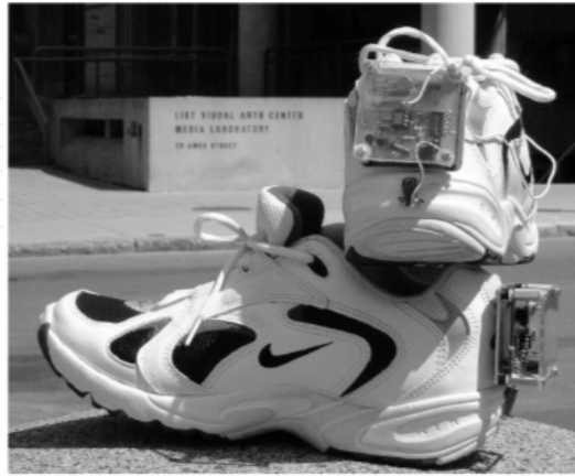
Figure 2. Piezoelectric-powered RFID shoes with mounted electronics.
