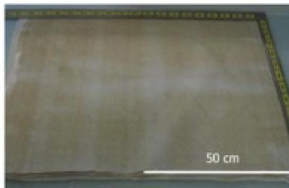
**Figure 11.** Visual examination of a fouled NF membrane
