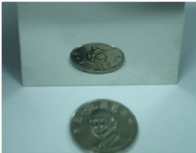
Figure 2. The image of the mirror-like 304 stainless steel substrate after the EP process.
