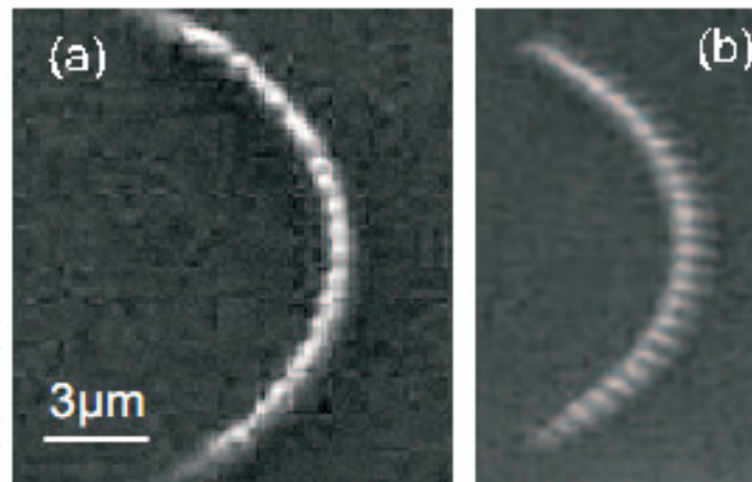
Figure 33. Scanning electron microscope (SEM) (a) the top image of the structure, (b) the image of the structure obtained with view angle 45^\circ . The radius of curved chains of nanoparticles is equal to 10\mu\text{m} . The particle in-plane size (diameter) and inter-particle distance are estimated to be about 350\text{nm} and 850\text{nm} , respectively, the particle height is 300\text{nm} . Reprinted with permission from “A. B. Evlyukhin, et. al, Opt. Exp. 15, 16667-16680 (2007).” of copyright ©2007 Optical Society of American.
