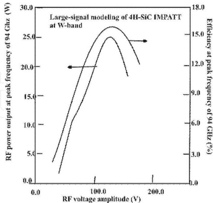
**Figure 6.** Plots of power generating efficiency and RF power with ac voltage amplitude of hetero-structure DDSiC IMPATTs for fundamental operating frequency 94 GHz (current density  $8 \times 10^8 \text{ Am}^{-2}$ )
