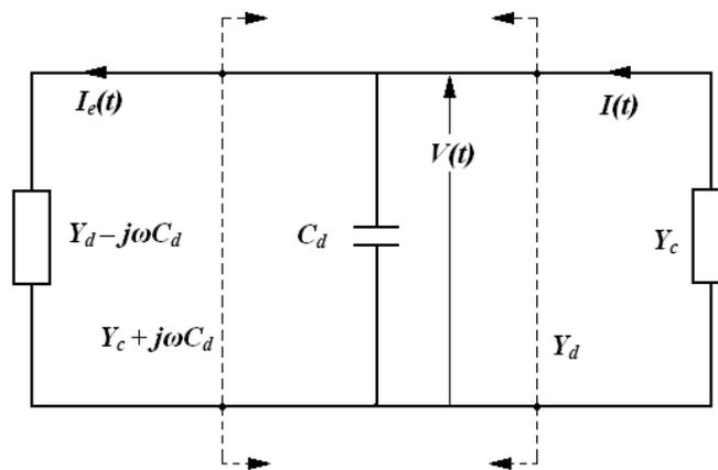
**Figure 2.** Terminal voltage and current for an IMPATT diode showing the separation of the depletion region capacitance  $C_d$  from the diode admittance  $Y_d$ .  $Y_c$  is the circuit admittance including the diode package.
