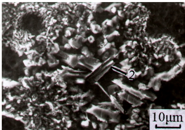
Figure 19. Fine flaky iron-rich phase indicated by arrow 2 appears in DEASA (EZL108) containing iron level of 0.25%.
