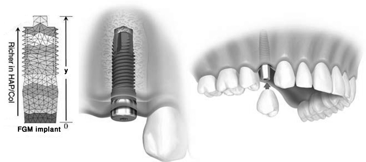
Figure 1. Schematic view of FGM dental implant with graded material composition.
