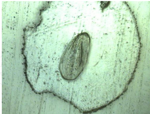
Figure 9. Cross-section of trabecula embedded in epoxy resin. Image acquired by optical microscopy.
