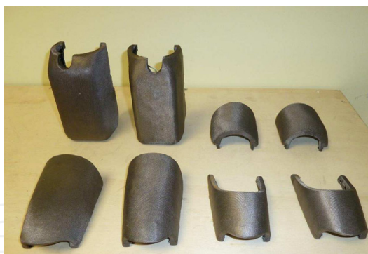
Figure 14. The covers of iCub arms covered with conductive lycra
