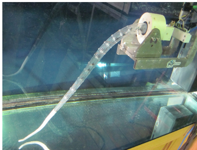
Figure 11. The SMA-based tentacle (See http://www.octopusproject.eu/ ).
