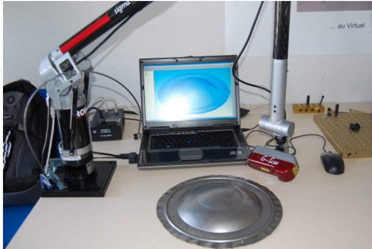
Figure 9. 3D scanner G Scan for reconstitution
