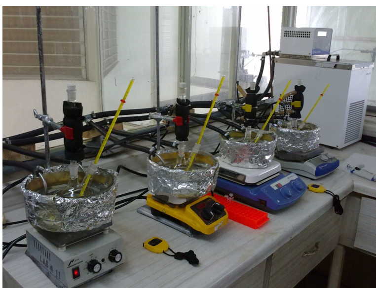
Figure 8. Transesterification reaction system for the conventional process
