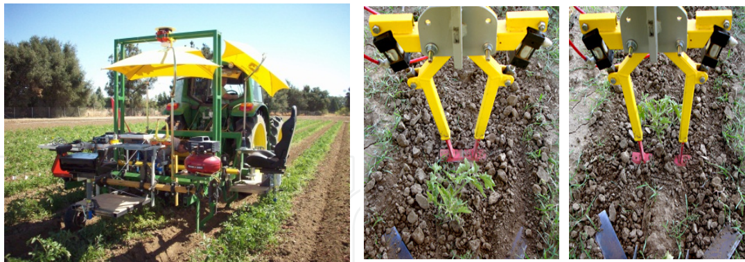
Figure 16. A RTK-GPS based robotic cultivation system-(a) A cultivator retrofitted with a RTK-GPS system in operation, and (b) The cultivating tines open to protect the plant based on the plant map and closed to get rid of weeds in between plants in the crop row.
