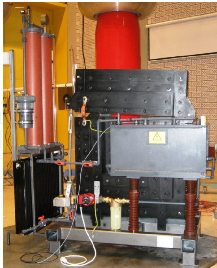
Figure 9. The resonant coil - a key ICAAS component
