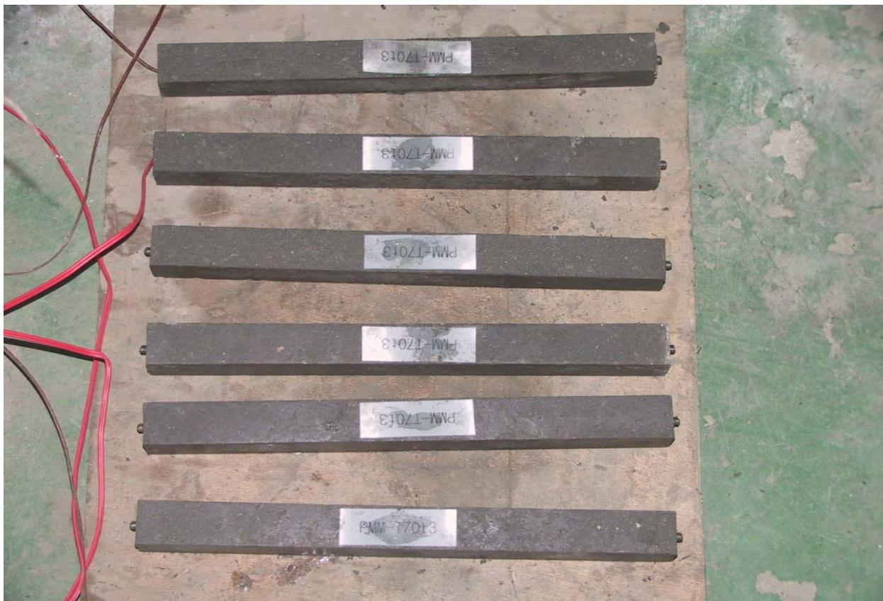
**Figure 4.** Strain gage setup for length change
