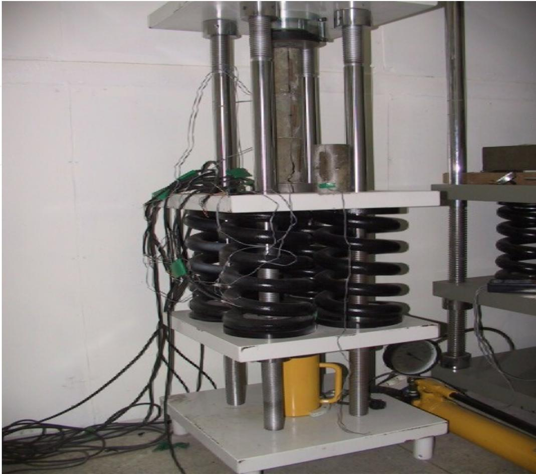
**Figure 5.** Compressive creep test
