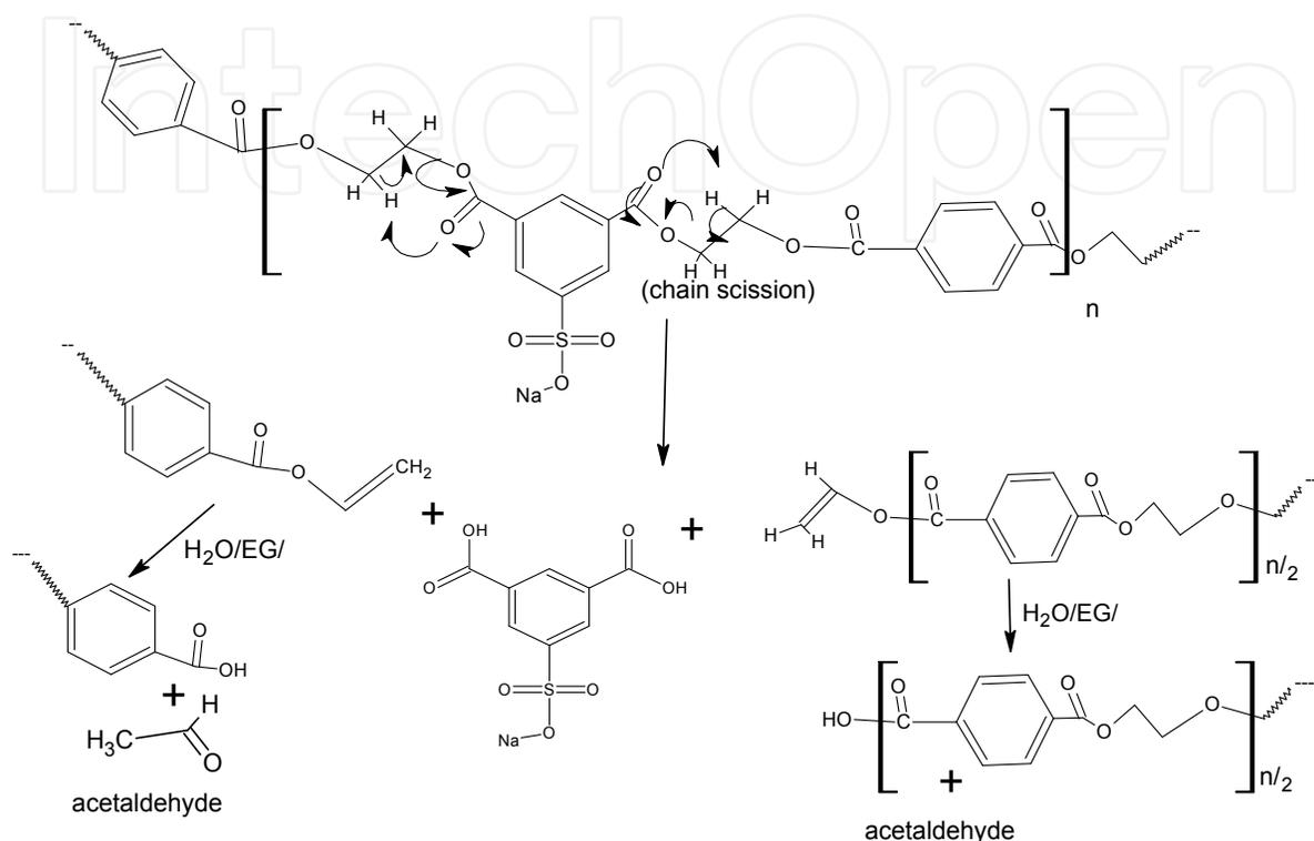
**Scheme 11.** Mechanism of degradation of polymer containing
