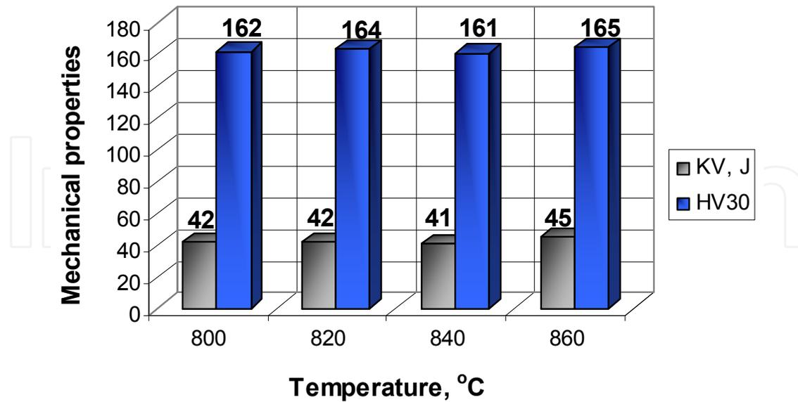
**Figure 16.** Change in the values of hardness and impact energy of the cast steel depending on the temperature of  $(\alpha + \gamma)$  annealing
