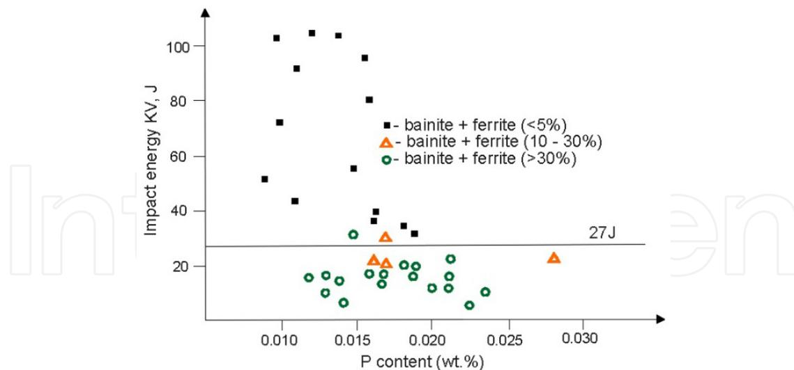
**Figure 3.** Influence of phosphorus amount and microstructure on impact energy KV of the Cr – Mo – V cast steel after long-term operation at the temperature of 535 °C
