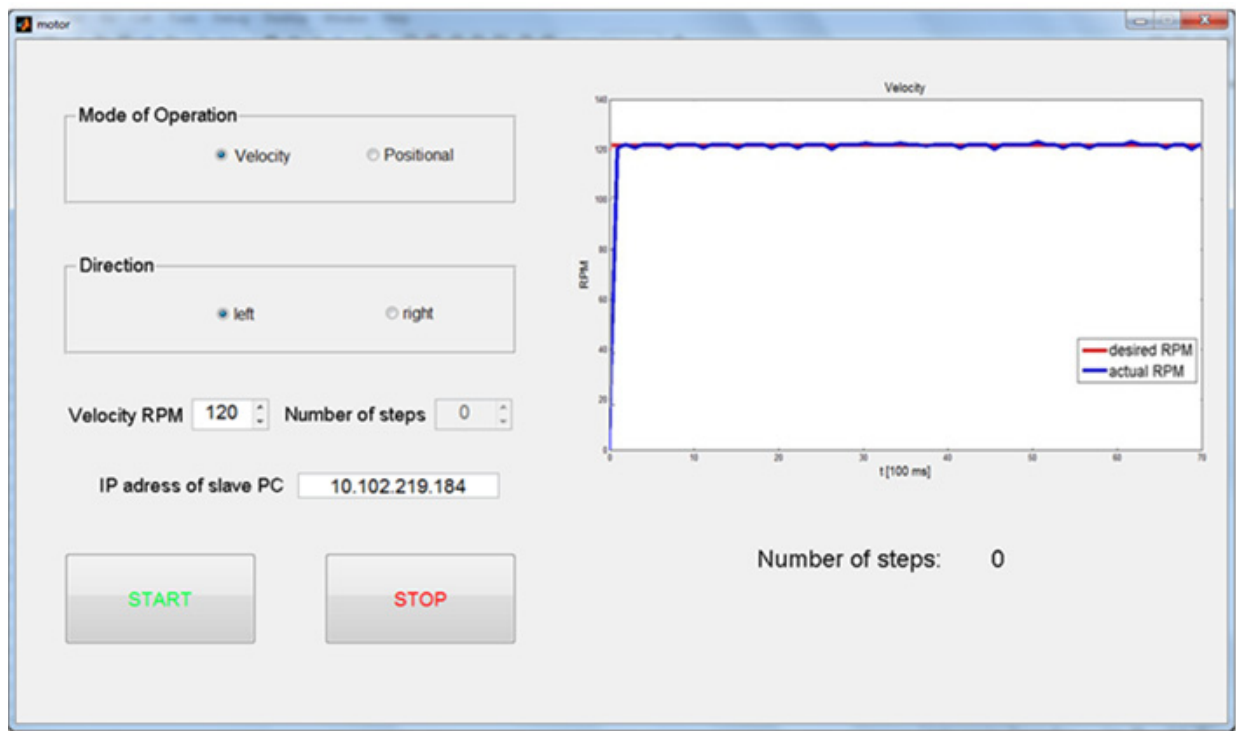
Figure 11. Graphical User Interface for stepper motor system
