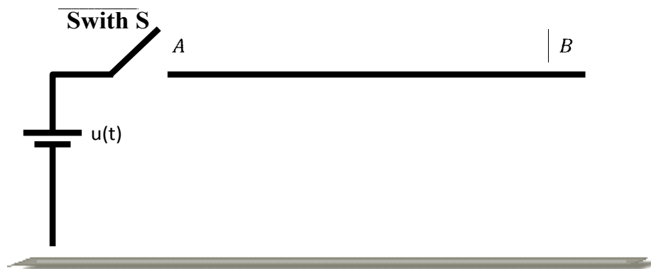
Figure 11. Single phase line representation with opened terminal.
