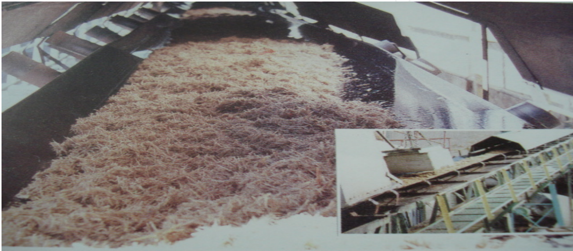
Figure 4. Transported the Bagasse through the conveyer belts from the sugarcane factory to the paper factory
