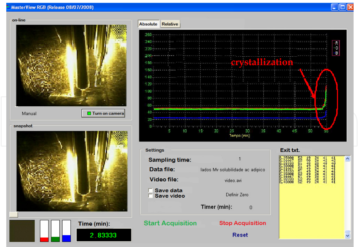
Fig. 9. Monitoring of the onset of the crystallization of adipic acid using the image analysis method (increasing the mass of adipic acid crystals due to cooling).
