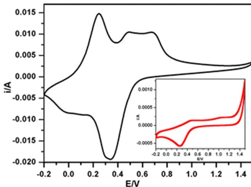
**Figure 3.** Cyclic voltammogram of PSC and inset shows the cyclic voltammogram of PANI in H<sub>3</sub>PO<sub>4</sub> medium at a scan rate of 20 mV/s.
