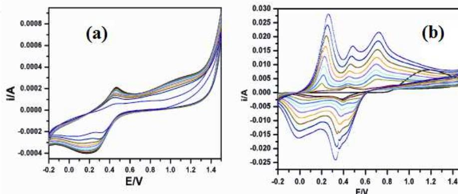
**Figure 2.** Electrochemical growth behaviour of (a) 0.1M aniline in 0.2M H<sub>3</sub>PO<sub>4</sub> medium and (b) aniline- SiO<sub>2</sub> in 0.2M H<sub>3</sub>PO<sub>4</sub> medium in potential range between -0.2 V to 1.5 V vs. Ag/AgCl at scan rate of 20 mV/s.
