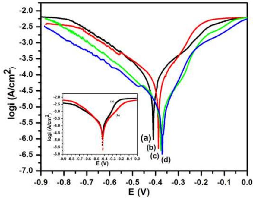
**Figure 8.** Tafel curves of PANI coated mild steel electrode with different loading level of PANI in epoxy resin (a) 1.5% (b) 3.0% (c) 4.5% (d) 6.0% whereas the inset shows (a) blank mild steel electrode and (b) epoxy coated mild steel electrode in 1.0 M HCl.
