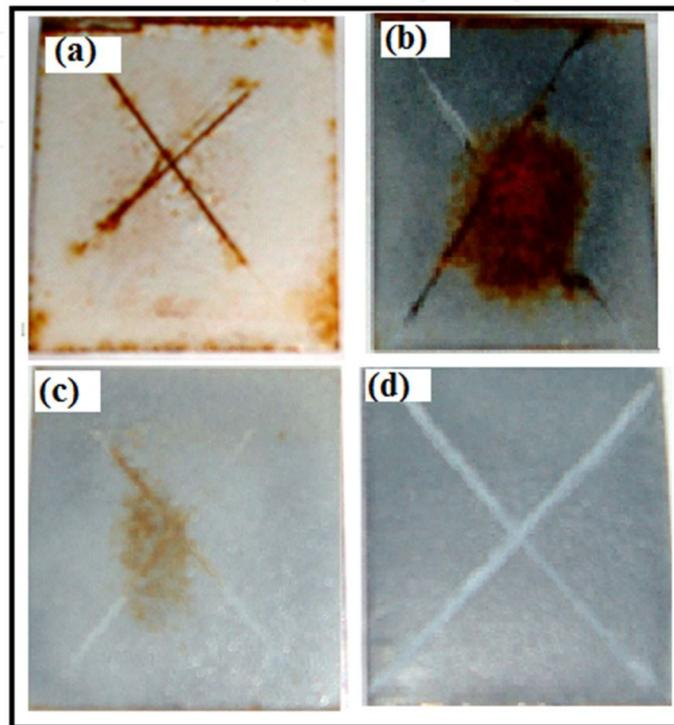
**Figure 21.** Photograph of (a) epoxy coated (b) PANI (at 6 wt.% loading) coated (c) HPSC (at 1.5 wt. % loading) and (d) HPSC (6.0 wt. % loading) mild steel after 35 days of exposure to salt spray test.
