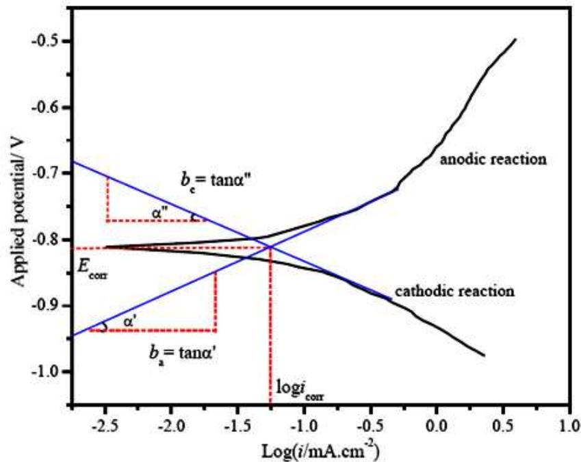
**Figure 1.** Schematic polarization curve showing Tafel extrapolation.
