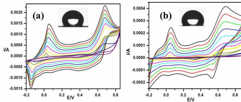
**Figure 14.** Electrochemical growth behaviour of (a) 0.1M aniline in 0.2M PFOA medium and (b) aniline- SiO<sub>2</sub> in 0.2M PFOA medium in potential range between -0.2 V to 0.9 V vs. Ag/AgCl at scan rate of 20 mV/s.
