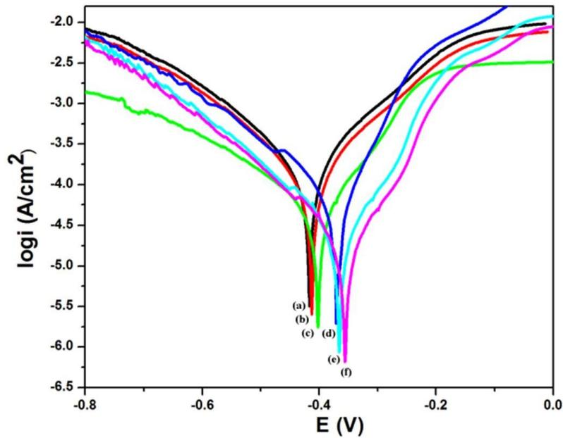
**Figure 18.** Tafel curves of uncoated and polymer coated mild steel electrode in 3.5 % NaCl solution (a) blank electrode (b) epoxy coated mild steel (c) PANI coated mild steel at 1.5 wt. % loading (d) 3.0 wt. % loading (e) 4.5 wt.% loading and (f) 6.0 wt. % loading of PANI in epoxy resin.
