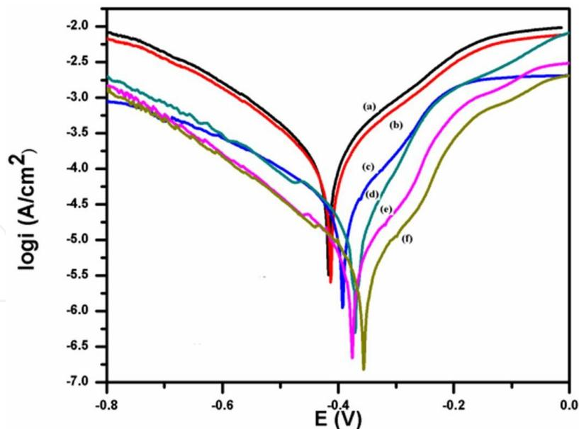
**Figure 19.** Tafel curves of (a) blank mild steel (b) epoxy coated mild steel (c) HPSC coated mild steel at 1.5 wt. % loading (d) 3.0 wt. % loading (e) 4.5 wt.% loading (f) 6.0 wt. % in 3.5 % NaCl solution.
