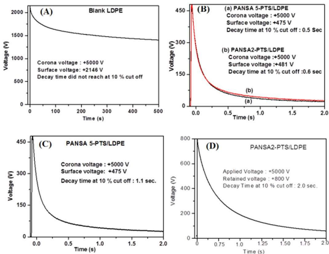
**Figure 30.** ESD-graphs of LDPE film in the presence of AN-ANSA copolymers (A) blank LDPE film, (B) Copolymer/LDPE nanocomposites film at 1.0 wt.% loading, (C) PANSAs 5-PTS at 0.5 wt. % loading and (D) PANSAs 2-PTS at 0.5 wt. % loading (Reproduced with permission from Ref. 77, Copyright 2009 John Wiley & Sons).
