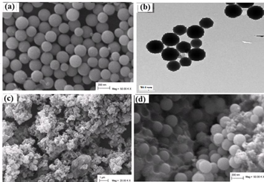
**Figure 10.** SEM micrographs powder sample of (a) SiO<sub>2</sub> (c) PANI (d) PSC and (b) TEM image of SiO<sub>2</sub> particles.
