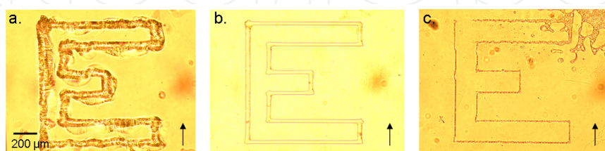
Figure 8. Letter "E" patterns (a) by one-photon photopolymerization (UV irradiation) in a nonaligned sample, (b) by one-photon photopolymerization (UV irradiation) in an aligned sample, (c) by two-photon photopolymerization (IR irradiation) in an aligned sample. The nematic director orientation is indicated by the arrow.
