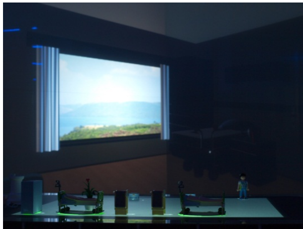
Figure 3. The room layout configurator. The foreground shows the surface table with tangible objects. The background shows the wall display with the virtual room.
