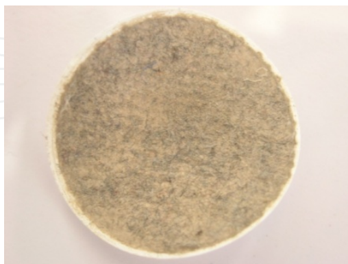
Figure 1. Non-dissolved particles captured on the filter
