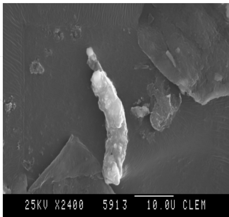
Figure 7. Detail of various shapes of settled particulate matter
