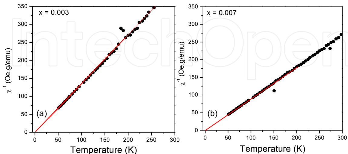
**Figure 9.** The temperature dependence on the inverse of susceptibility, recorded at 100 Oe, shows low temperature paramagnetic character for  $\text{Pb}_{1-x}\text{Mn}_x\text{S}$  NCs embedded in borosilicate glass matrix.
