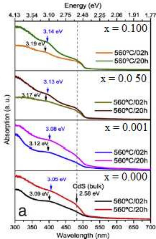
**Figure 5.** Panel (a): Room-temperature OA spectra of  $\text{Cd}_{1-x}\text{Mn}_x\text{S}$  NCs embedded in SNAB glass matrix with concentration  $x = 0, 0.001, 0.050,$  and  $0.100$ . The well-defined sub-band peaks demonstrate quantum confinement regimes and the relatively narrow dot size distributions. The energy shift of the OA peaks indicates the Mn incorporation in the dots.
