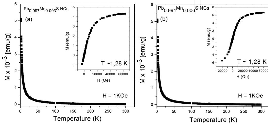
**Figure 10.** Magnetization as a function of temperature for the  $\text{Pb}_{0.997}\text{Mn}_{0.003}\text{S}$  and  $\text{Pb}_{0.994}\text{Mn}_{0.006}\text{S}$  NCs embedded in borosilicate glass matrix. Field dependence of magnetization for each sample is shown in the insets.
