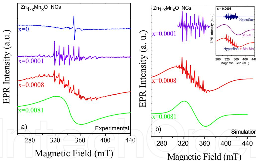
**Figure 6.** (a). Room-temperature X-band EPR spectra of  $\text{Zn}_{1-x}\text{Mn}_x\text{O}$  nanocrystals at different  $x$  values and (b) Simulated EPR spectra of  $\text{Zn}_{1-x}\text{Mn}_x\text{O}$  nanocrystals for different  $x$  values. In inset illustration of processes used for EPR spectra simulation of the  $\text{Zn}_{1-x}\text{Mn}_x\text{O}$  nanocrystal ( $x = 0.0008$ ).
