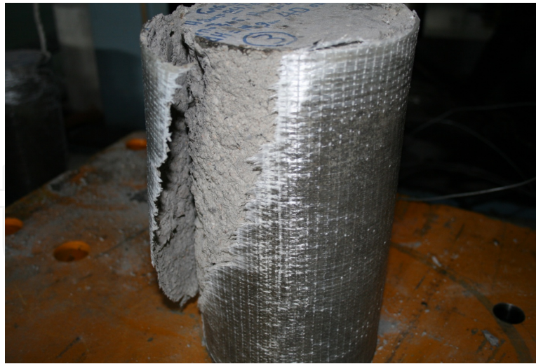
Figure 7. Specimen of C16 concrete confined by 1 layer of GFRP and 3 layers of tPPFR material after the removal of the fiber rope. View of the GFRP fracture far from the overlap region.
