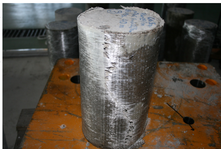
Figure 6. Specimen of C16 concrete confined by 1 layer of GFRP and 3 layers of tPPFR material after the removal of the fiber rope. The GFRP sheet jacket is fractured in two opposite positions. View of the fracture near the overlap region.
