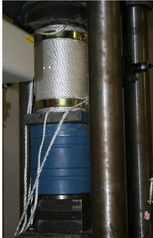
Figure 5. Test setup of specimens confined by 1 layer of GFRP and 3 layers of tPPFR material.
