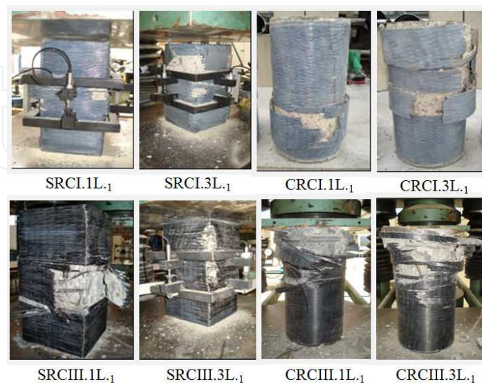
Figure 11. Typical failure modes for the tested specimens
