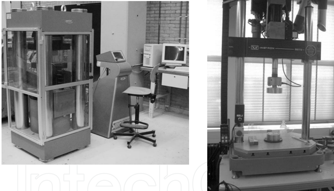
Figure 4. Experimental testing device for concrete compression (Left) and tension (Right).
