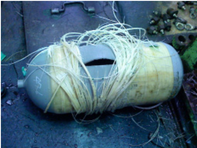
Figure 4. Composite vessel after burst test
