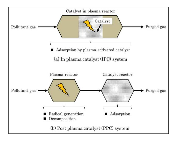
**Figure 9.** Typical process flow diagrams and description of main functions of Post Plasma Catalyst (PPC) and In Plasma Catalyst (IPC) system [55, 56].
