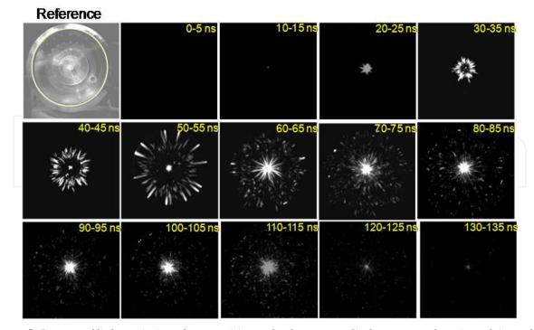
**Figure 6.** Images of light emissions from positive pulsed streamer discharges as a function of time after initiation of the discharge current.
