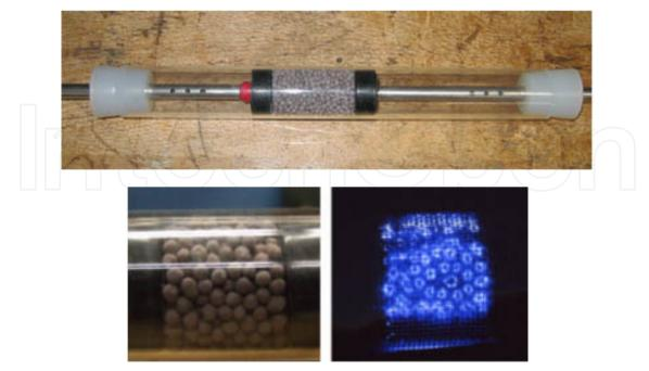
**Figure 10.** Schematic diagram and its appearance of packed-bed reactor (Photograph: Prof. Takaki group, Iwate University, Japan)[50], [53].
