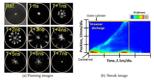
Figure 8. Framing and streak images of nanoseconds pulsed discharge in a coaxial electrode..
