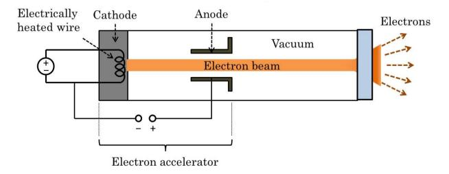
Figure 2. Schematic representation of electron beam source.
