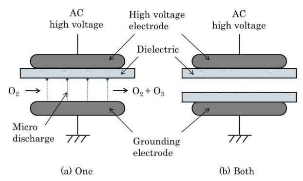
Figure 4. Schematic representation of dielectric barrier discharge electrode.
