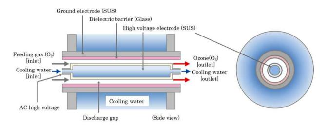
Figure 5. Schematic representation of cylindrical cooled reactor.
