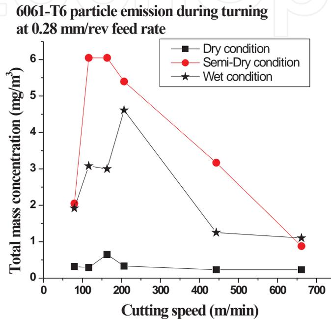
Figure 21. Total mass concentration at different lubrication conditions
