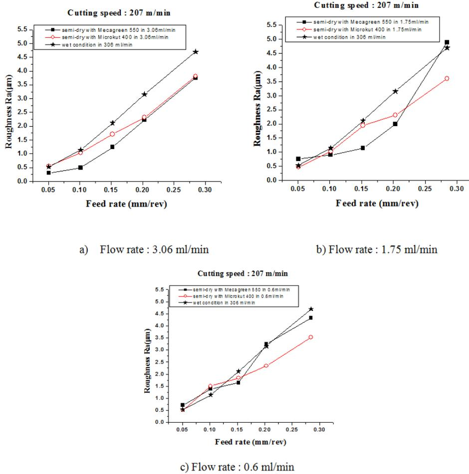
Figure 9. Lubrication debit comparison on the roughness during turning process of 6061-T6 at the same cutting speed using Mecagreen 550 and Microkut 400 lubricant
