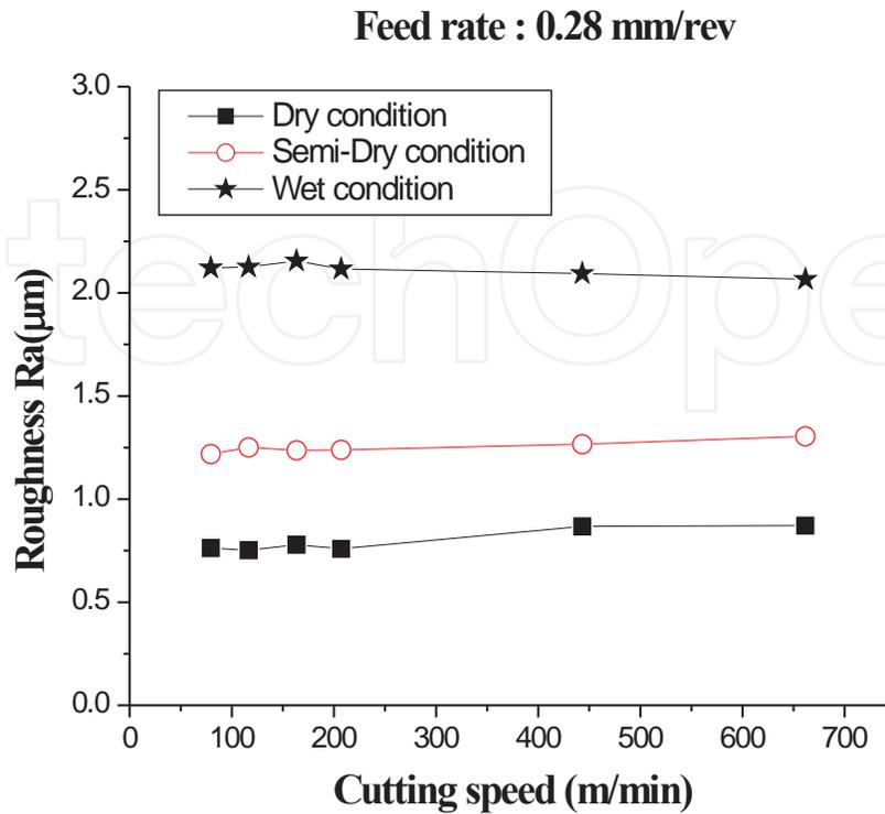
**Figure 5.** Roughness against cutting speed
