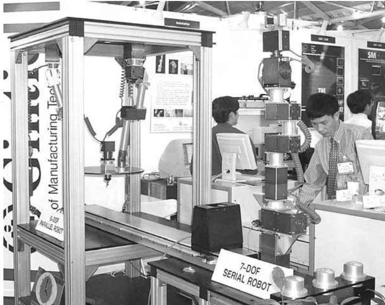
Figure 15. A light machining workcell with modular robot components
