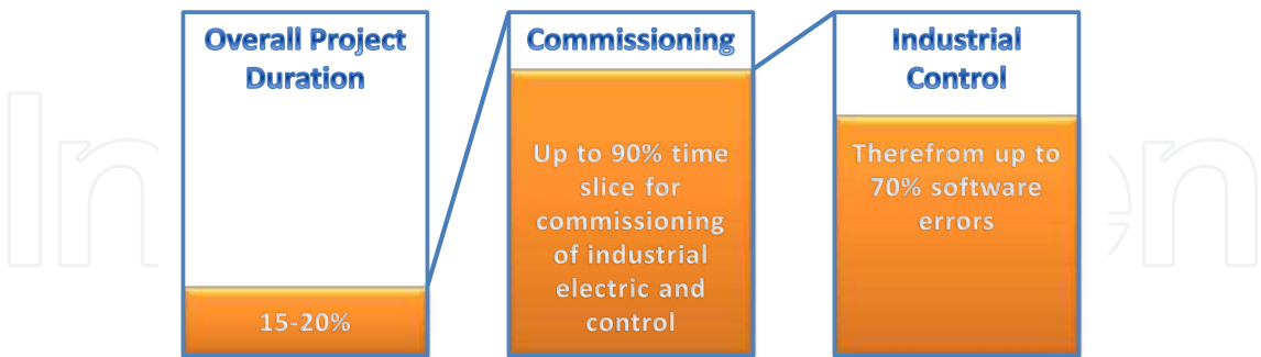
Fig. 2. Contribution of control software to project delay (Wunsch, 2008)
