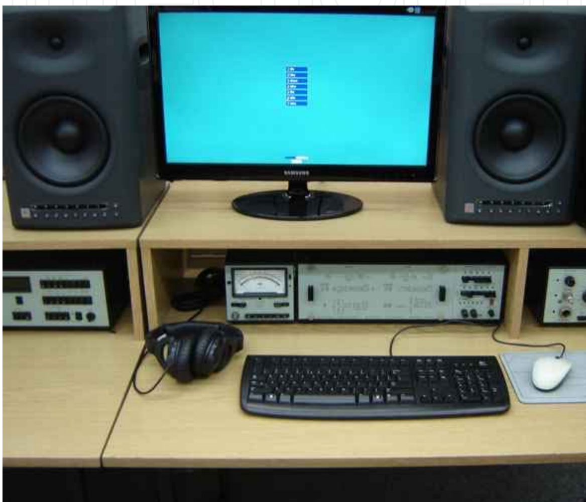
Fig. 9. Speech quality subjective measurement stand.
