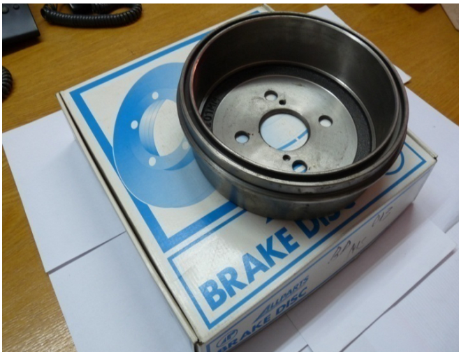
Figure 47. A Brake Drum made by PM process.
