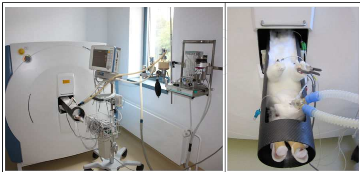
Figure 2. \mu -computed tomography of the rabbit tibia under general anaesthesia.
