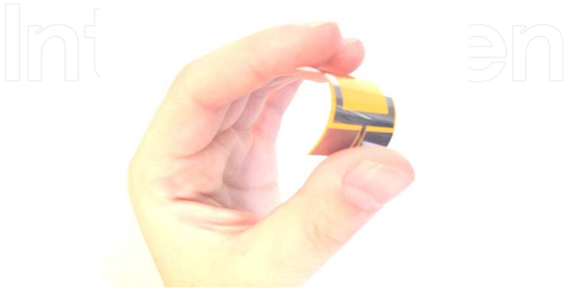
Figure 1. Flexible printed monopole antenna based on Kapton Polyimide substrate.
