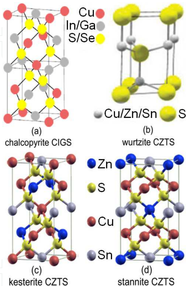
Figure 4. Crystal structures of CIGS and CZTS [13, 14].
