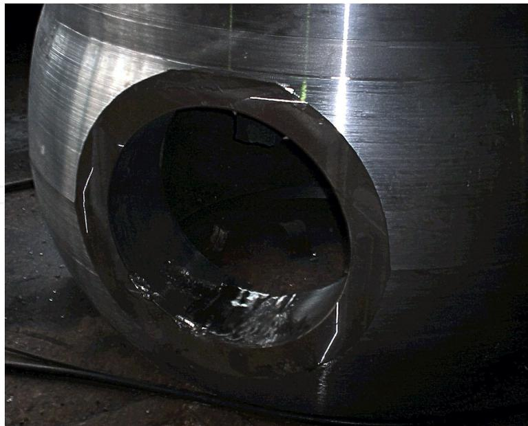
**Figure 30.** Casting defects in the block window.
