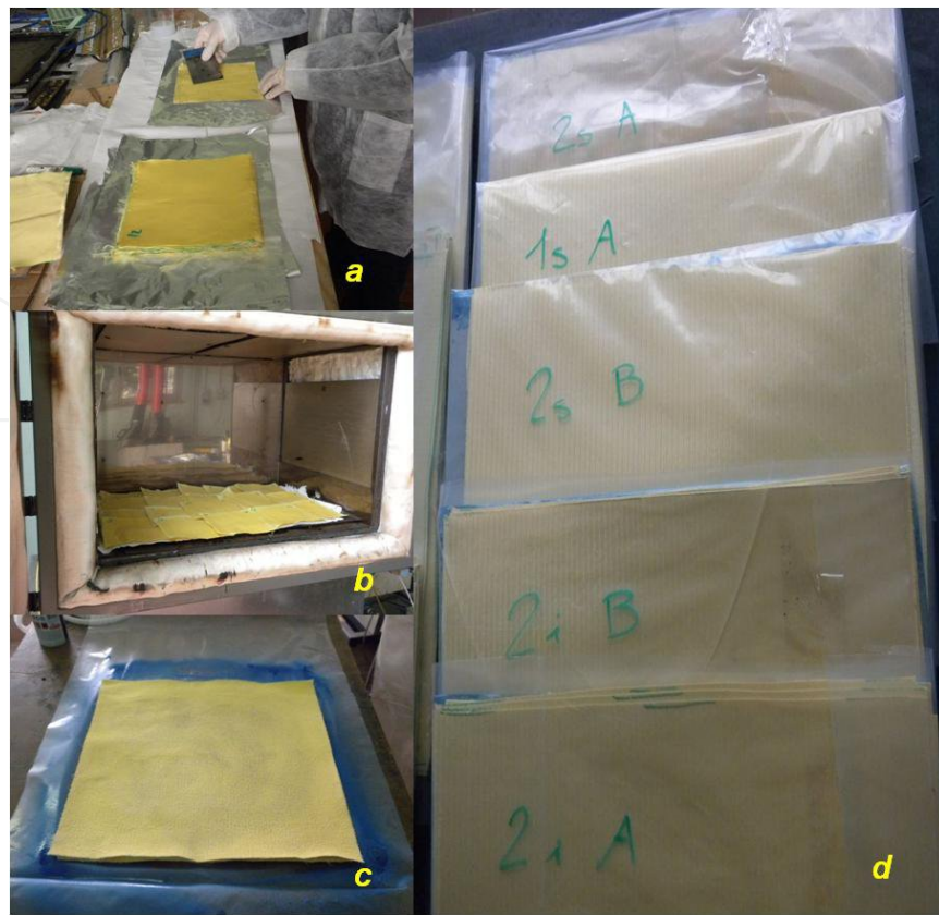
Figure 6. Different step of Kevlar-reinforced based antiballistic panels manufacturing: a) fluid application onto layers surface, b) solvent evaporation in oven, c) enveloping procedure, d) the panels ready for the ballistic test.
