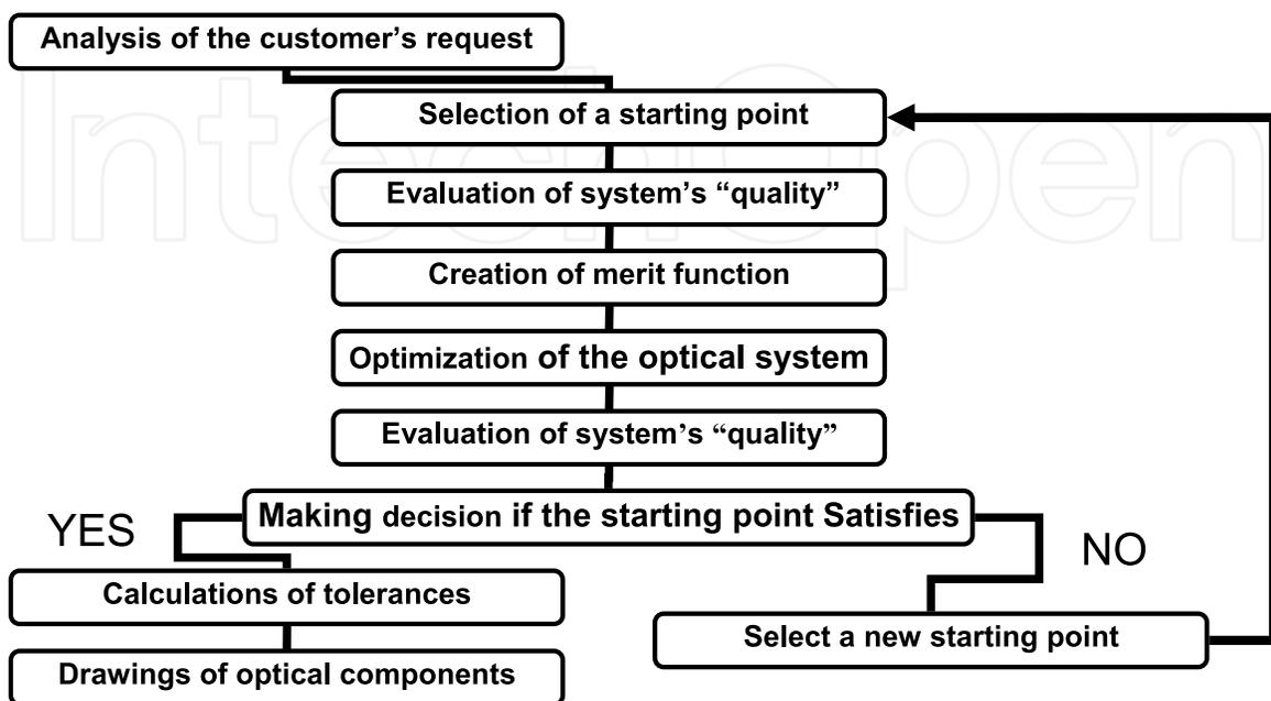
Fig. 3. Stages of the optical design procedure
