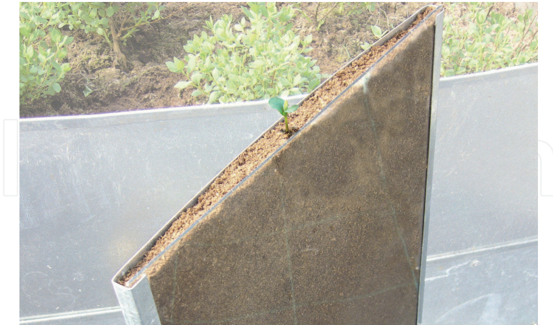
Fig. 7. The root box constructed from a metal frame and glass front wall used for the analytical assessment of the root growth and structures (Drobná, 2010).
