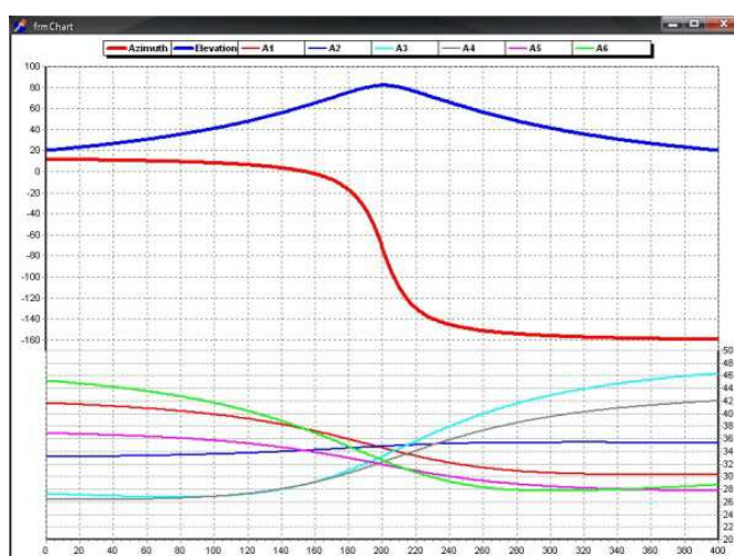
Fig. 16. Graphs of the aimer table transformation in the topocentric coordinate system ( \mathbf{R}[t_j, \alpha_j, \beta_j] ) and in the local coordinate system \mathbf{R}[t_j, \alpha_{1j}, \alpha_{2j}, \alpha_{3j}, \alpha_{4j}, \alpha_{5j}, \alpha_{6j}] .
